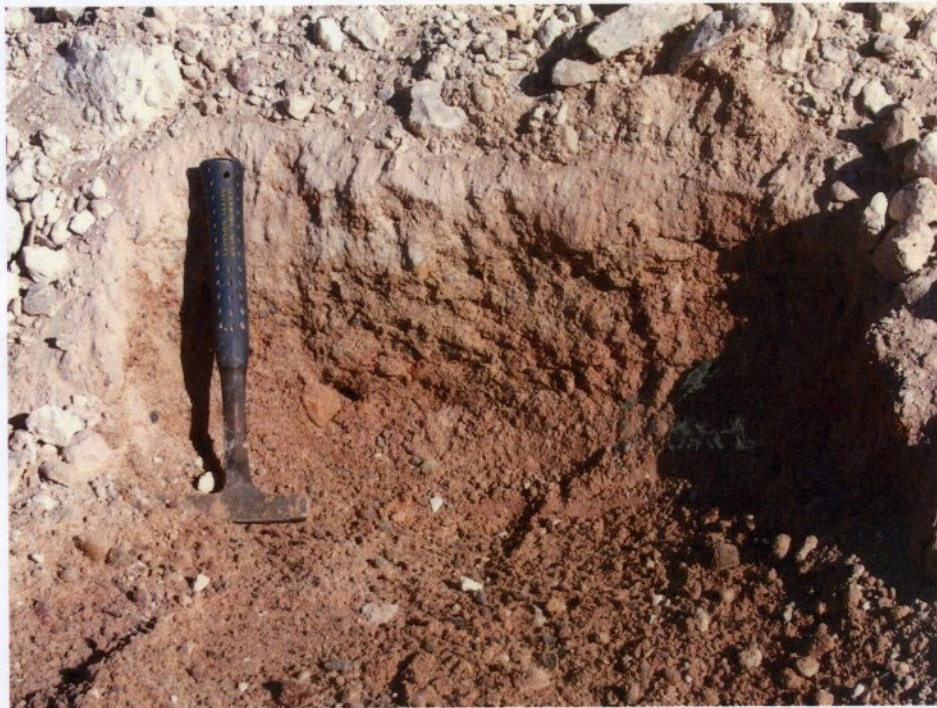
Photo 6 Moist OAG along north excavation wall; dry material is lighter color (Diane Poteet photo)
